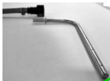
NH 3 -line from ASDS entering SCRT via 1/4" steel pipe
